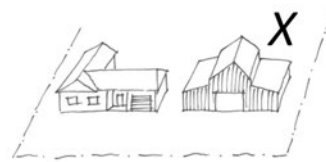
Figure 7- Inappropriate bulk and height of the outbuilding
