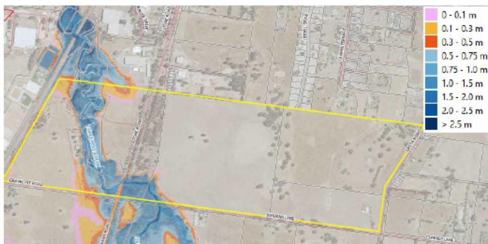
Figure 5 Area Wang W1-C (north-west) – Wangaratta flood study 1% AEP depth mapping along Three Mile Creek breakout along Reith Road to the south of Shanley Street
